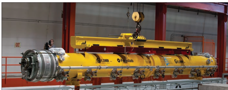
When complete, the prototype accelerator will comprise six cryomodules like this first example. Each weighs about 8 tonnes and contains eight SRF cavities. (Courtesy Fermilab Visual Media Services.)
